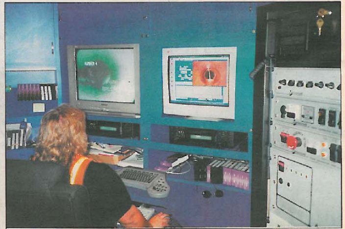
Top left: Joyce Taylor Velitschkowski, founder and owner of JTV, Inc., with one of her custom-built video inspection vehicles. Top right: JTV crew with a specially-equipped combination vehicle for large diameter pipe cleaning projects. Above left: Joyce and crew video inspect a lateral prior to lining. Above right: Joyce conducts a pipe survey using a Pearpoint mainline camera in conjunction with flexidata pipe survey reporting software.
